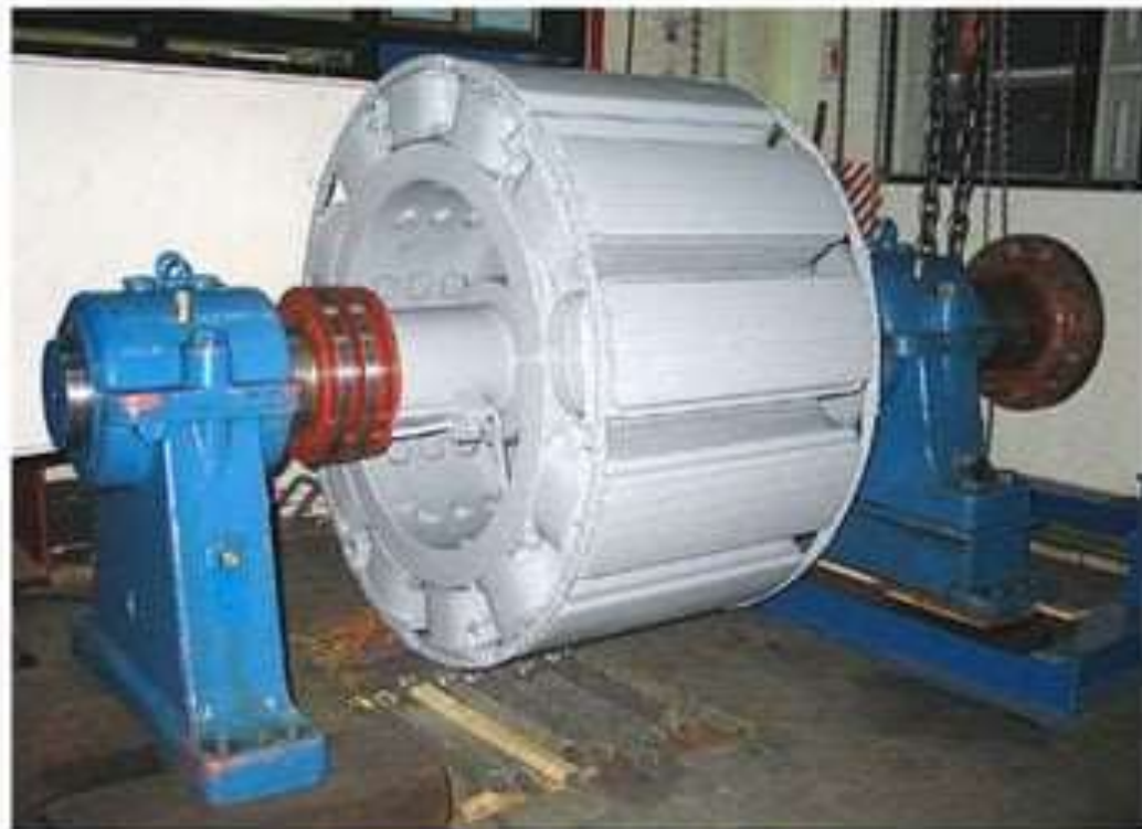
HABU POWER STATION (UNIT 2), MALAYSIA UPRATING OF 11 KV, 2.5 MW HYDRO GENERATOR TO 2.75 MW COMPLETE 'H' CLASS REINSULATION OF ROTOR POLES
